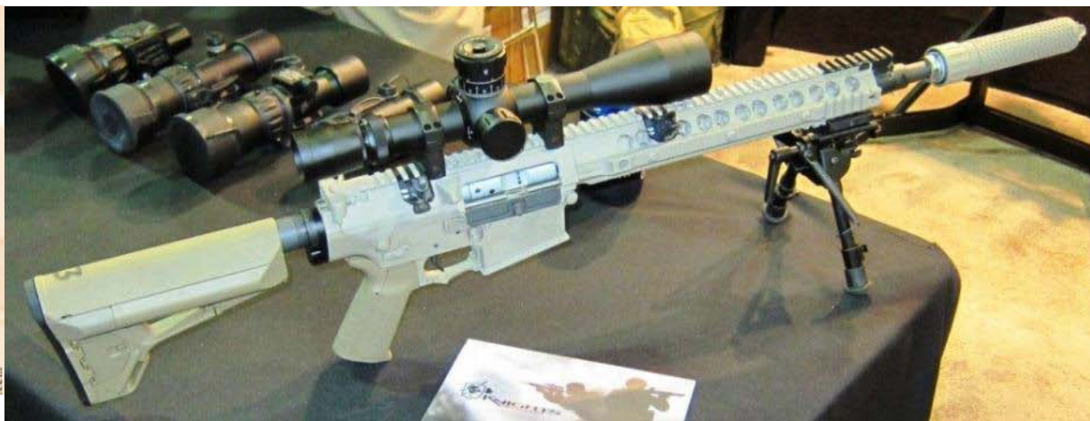
Knight's Armament M110C (Carbine) Configuration – Army has indicated interest in such a system. M110C Weight is 8.9 lbs unloaded without optic or 762 QDC suppressor (has 16 inch Chromed Barrel)
