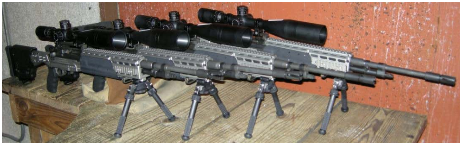
MK 14 MOD 2 EBR – EDMV Systems at the Underground Range Bench B&T Industries BT10 Atlas Bipod is used (alt. feet and leg extensions avail.) Magpul PRS 2 Buttstock is used with Sage Adj. Height Buttpad Interface.
