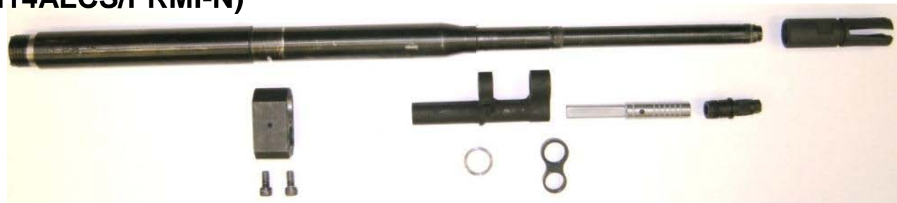
The M14 SSR Full Heavy Profile Match Barrel (1 in 10 inch twist) remains, but most associated parts get replaced w/ Sage Op. Rod Guide, SEI Gas Cylinder, Chromed Piston, and Vortex DC Flash Suppressor.
