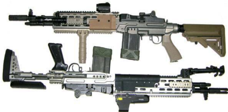
Sage MK 14 Mod 1 Chassis w/ Crane Buttstock & Compact Reflex Sight and ACLS (Mod 0) Below
