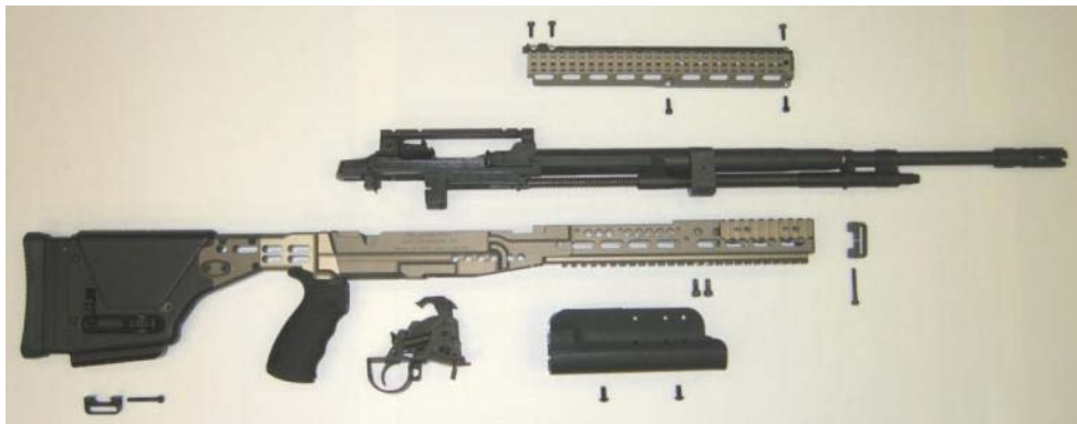
MK 14 MOD 2 Barreled Action Separated from Sage Chassis Stock (PN M14ALCS/PRMI-N)
