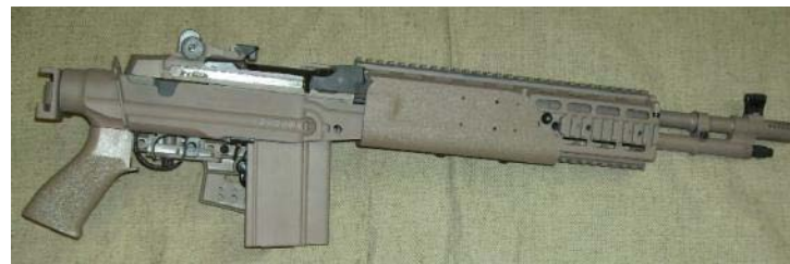
Folding Buttstock Adapted Sage Chassis System with 16 inch SAI Barrel
