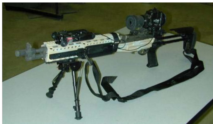
Lightened Prototype Stock with 16 inch barrel, modified SAI (Springfield Armory Inc.) Brake & Mini Night Vision Sight (AN/PVS-17) in Prototype Mount (2003)
