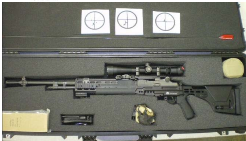
M14 EBR-RINM Prototype Kit – Medium Wt. SEI Configuration Barrel, Magpul PRS-2 Buttstock on Sage Iron Sight Capable Interface
