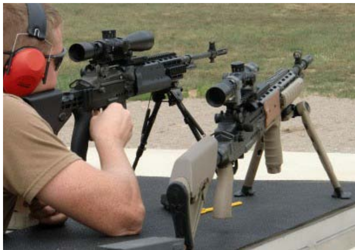
M14 EBR-RINM Prototype Kit – Medium Wt. SEI Configuration Barrel, Magpul PRS-2 Buttstock on Sage Iron Sight Capable Interface
