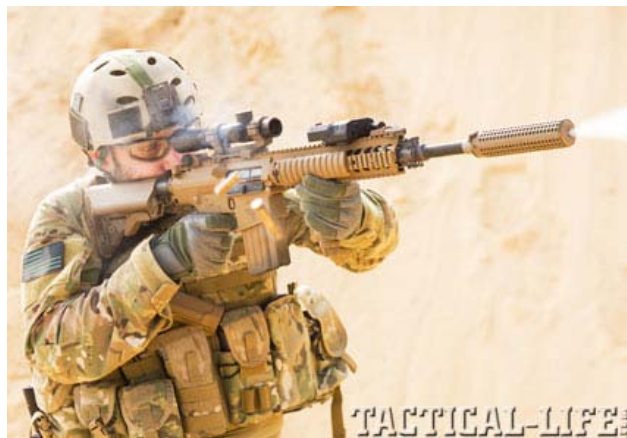
Knight's Armament M110C (Carbine) Configuration – Army has indicated interest in such a system. M110C Weight is 8.9 lbs unloaded without optic or 762 QDC suppressor (has 16 inch Chromed Barrel)
