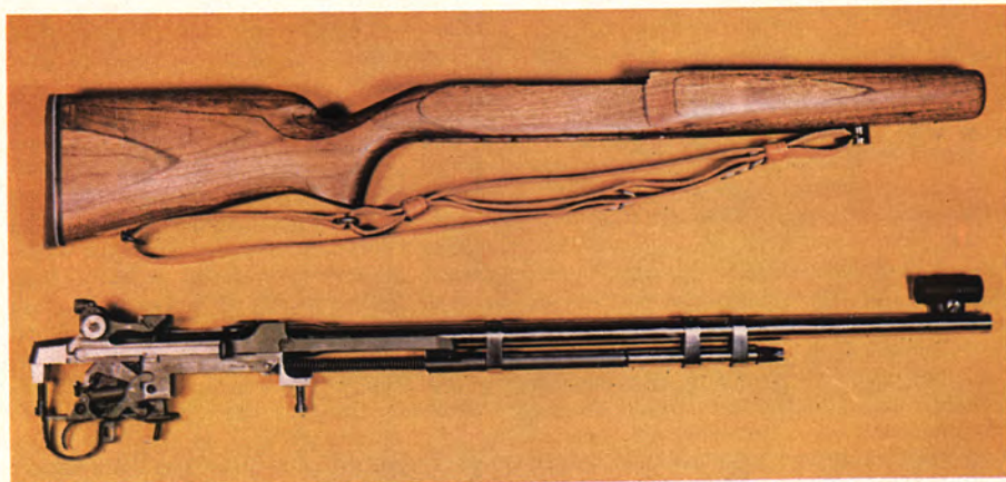
Prototype M14 National Match Product Improved Rifle, shown above assembled with sling and magazine, and below with stock removed to show details of barrel and gas system. Note absence of handguard.
