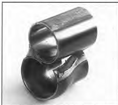
Steel shot fired through the lower barrel of a Winchester Model 101 over-under broke the soldered joint between the two barrels.
