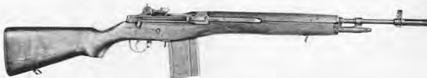
7.62 mm. Rifle T44E6, a shortened and lightened form of the M14, tested in 1958. T44E6 features are aluminum magazine (applicable also to M14 rifle if desired); barrel 2" shorter and somewhat lighter, and flash suppressor shorter, than M14; no gas spindle valve (this rifle was not designed to fire grenades); and no bayonet stud
