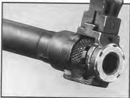
The flash hider is simply sawed off, welded and recrowned, while the bayonet lug is removed to satisfy the BATF.
