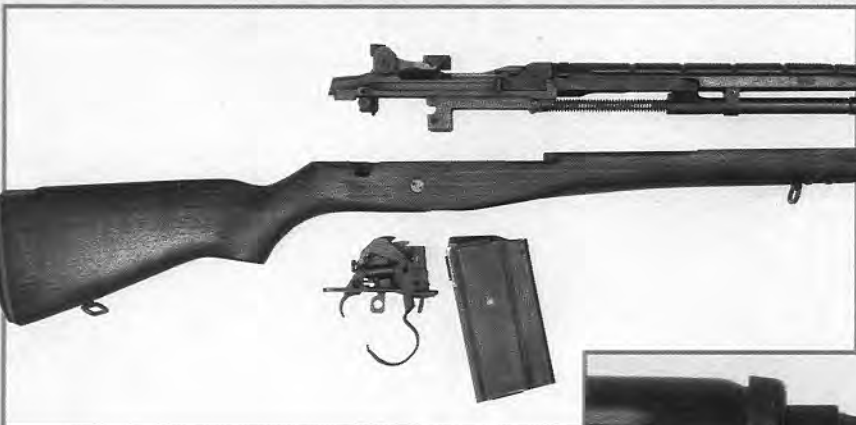
A simple flange at the rear of the gas cylinder stopped the M14's tendency to disassemble itself during Marine bayonet and wire-breaching exercises.
