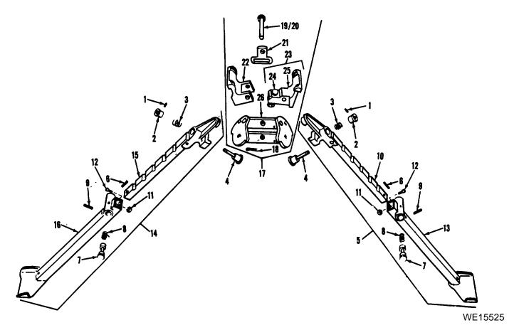
Figure 10. Rifle Bipod. M2- exploded view.
