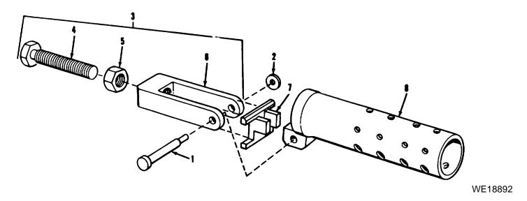
Figure 9. Stabilizer assembly- exploded view.
