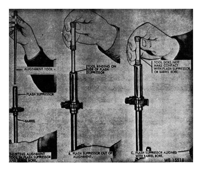
Figure 8-3. Checking alignment of flash suppresser with alignment tool.
