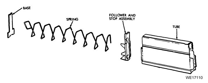
Figure 3-1. Magazine exploded view.
