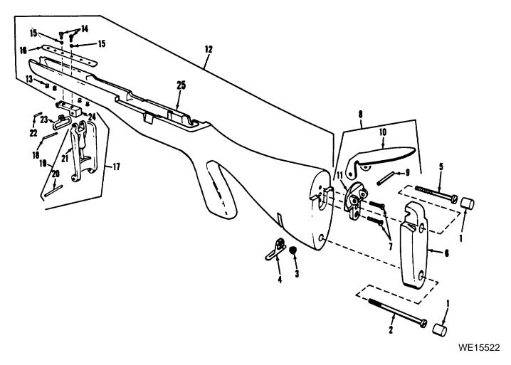
Figure 5. Shoulder gun stock assembly. Rifle, M14A1--exploded view.
