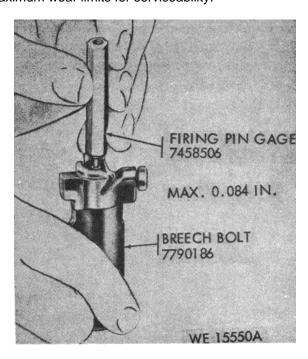
Figure 7-2. Checking diameter of firing pin hole.
