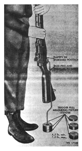
Figure 2-1. Trigger pull testing
