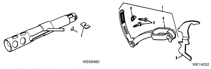
Figure 11. Combination tool-exploded view.
