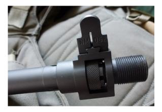
Once the rifle functioned reliably, I installed the suppressor and reduced (counterclockwise) gas pressure one-eighth of a turn at a time, when the rifle malfunction I stopped and increased gas pressure (clockwise) one-eighth. At this setting, the rifle worked reliably suppressed and unsuppressed. Furthermore, because M80 produces lower chamber and bore pressures than M118 or M118LR, you can be assured that your rifle will operate reliably across the full range of ammunition.
