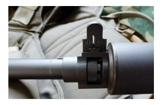
Unless you're a devotee of the M1A/M14 platform, it's very simple to overlook the gas shutoff originally designed into the rifle. It was used in support of rifle launched grenades -the Yugoslavian SKS took a similar approach - simply turn off the gas to prevent the weapon from cycling prior to launching a rifle mounted grenade.
