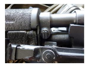
On the M1A/M14 you'll find the shut-off valve located on the starboard (right) side and aft (behind) of the gas plug. It looks like a set screw but functions like a ball vale. In the vertical position, gas is allowed to enter the gas cylinder. In the horizontal position, gas to the cylinder is shut off and the rifle will not cycle.
