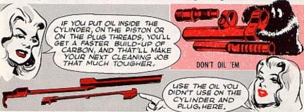
There're two places you don't want to forget to put oil. Those're the inside of the operating rod tube and the spring and plunger for the connector assembly. You get at the inside of the tube with an oily patch and your cleaning rod.
