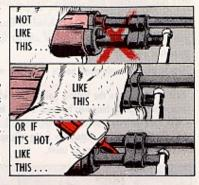
By the incidentally... that combination tool, FSN 4933-768-0211, is the only thing you want to use for removing and installing the gas cylinder plug. Use the combination tool to tighten the plug as tight as you can get it. Don't—double don't—use any extension on the tool for added leverage when you tighten the plug. The only time you might need extra leverage on the tool is when you go to remove a carboned-up plug.
