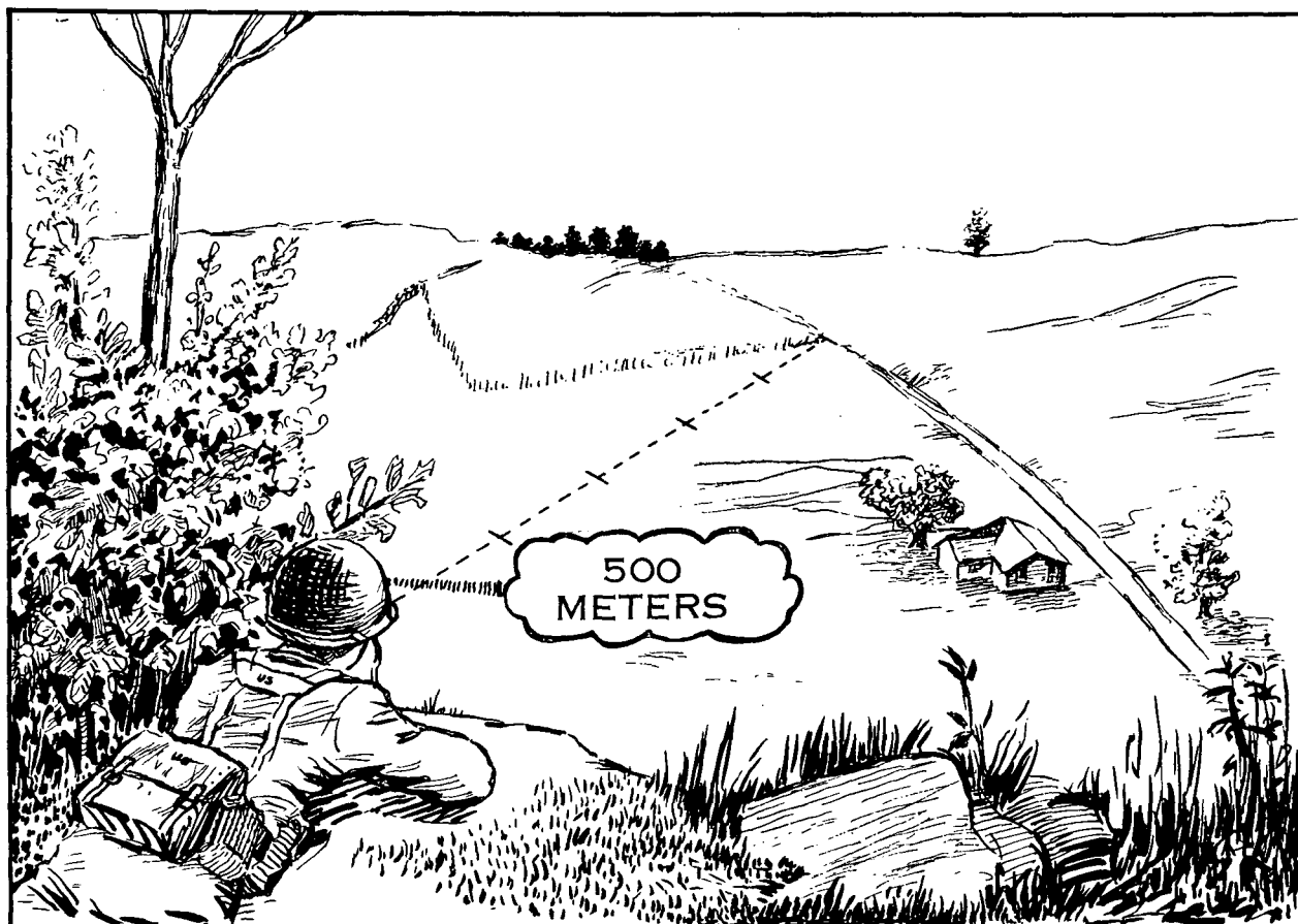
Figure 1. Applying the 100-meter unit of measure for ranges up to 500 meters.
