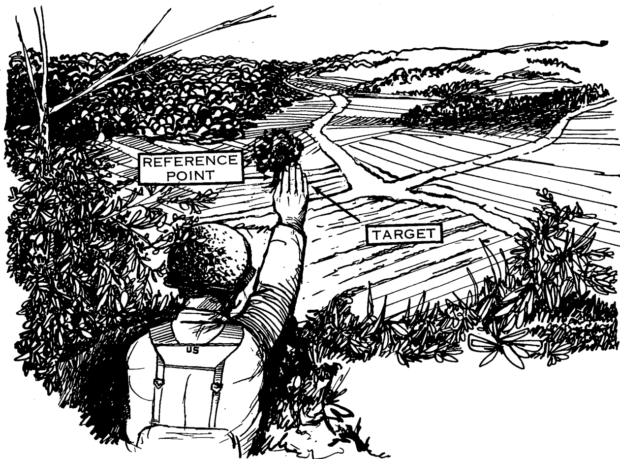
Figure 3. The finger measurement method.
